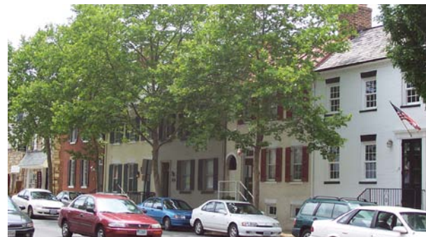
Image 4 - Where appropriate, neighborhood streets may be designed as 'yield streets' with curb to curb dimensions ranging from 28'-30', with parallel parking on both sides. The intent is to have cars 'queue' or 'yield' to each other as they pass by. Such streets may be appropriate when the length of the street does not exceed one or two blocks in length, when the fabric around it is of a low density such as single family detached homes and when the lots are served by an alley. Residential yield streets with parallel parking on both sides should have a design speed of 15-20 mph.
