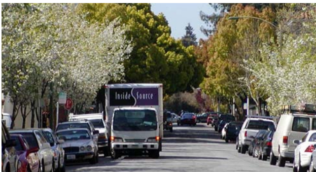
Image 3 - Principle neighborhood streets that connect one neighborhood to another may be designed as 'Free Streets', with curb-to-curb dimensions ranging from 32'-36' depending on their location, with two travel lanes, and parallel parking on both sides, and minimum 10' sidewalks. Residential streets with parallel parking on both sides of the street should have a design speed of 25-30 mph.
